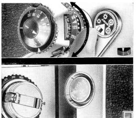
After placing the TTL Penta Prism in the camera turn the shutter-speed setting disc (51) once from stop to stop so that the driver pin (44) will engage the grooves on the bottom side of the TTL Penta Prism (45). This has been done correctly if, when the shutter-speed setting disc (51) is turned, the shutter-speed setting knob (10) is turning, too.
